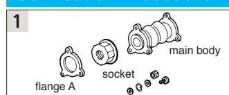
Remove the bolt and disassemble flange A and socket from the main body.
