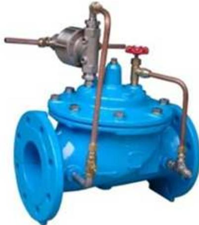
The Model 800 Differential Pressure Valve is a hydraulically operated, pilot-controlled, modulating valve. It is designed to maintain a constant pressure differential between any two pressure points in a system where the closing of the valve directly causes the differential pressure to increase. The valve tends to open on an increase in differential pressure and close on a decrease in differential pressure.
